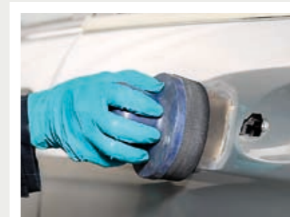
Apply Mirka guide coat to highlight imperfections on the surface.
