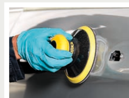
Remove paint from damaged area and feather out edges. Use Mirka grip disc P 80.
