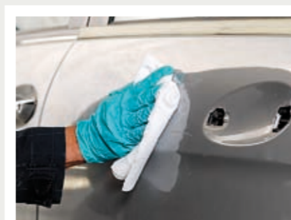
Preparation is key. Degrease the whole working area.
