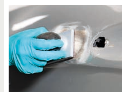
Re-apply Mirka guide coat. To further reduce scratch pattern use Mirka Abranet® strip P 180.
