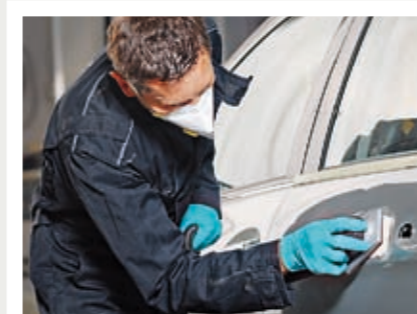
Hand sand filler area using Mirka Abranet® strip P 80.
